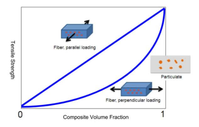
This demonstrates that the correlation is not linear for particulate composites, so while adding carbon fiber should add some strength, the parts will still be more akin to their original selves unless they get to over 75 to 80 percent Carbon Fiber. Since most filament composites are around 20% particulate, the difference in mechanical properties should be noticeable, but not substantial.
